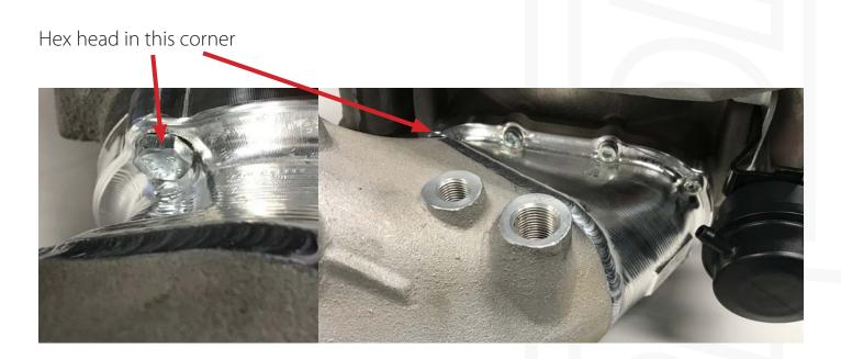
The upgraded assembly is now ready for installation of the baffle/core back into the manifold and then back on the vehicle. **Remember that if the bosses had to be ground on the underside when re installing the baffle/core into the manifold these screws will need to be assembled using Loctite 243 to ensure threads are sealed off and no boost pressure will be lost.**
