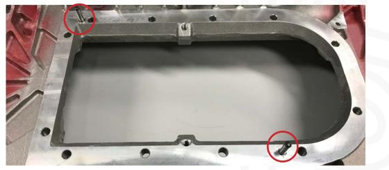
Fit the supplied O ring into the adaptor plate groove.
